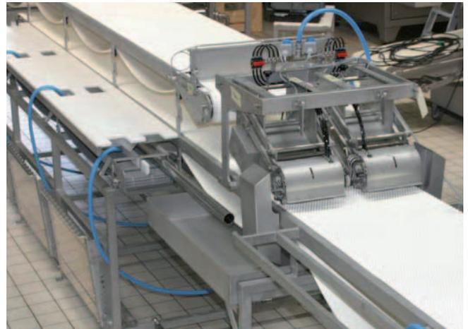
Pinbone section integrated into a trimming line
